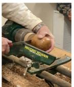
Use grain orientation/knots etc to determine the orientation of the finished piece.
